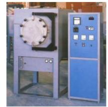
The dimensions of the chamber for the models FE-N are reduced around 10%. Standard electric supply V 380 triphase.
